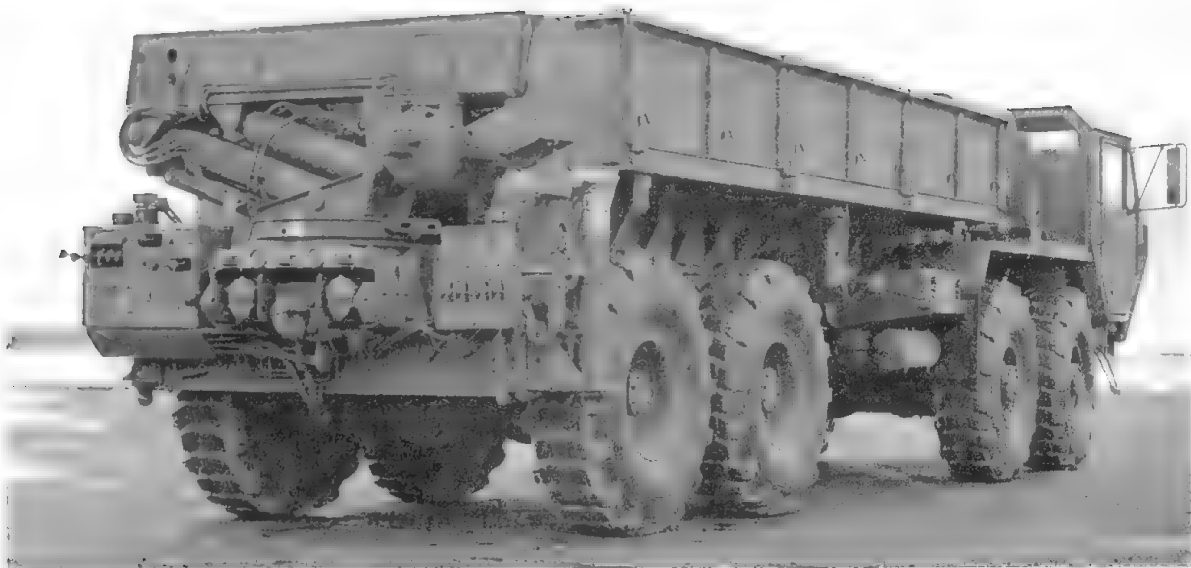
The knuckle-boom crane at the rear of the M977 HEMTT, along with its drop-side cargo body, makes the HEMTT a big improvement over previous military transports. (U.S. Army photo)
